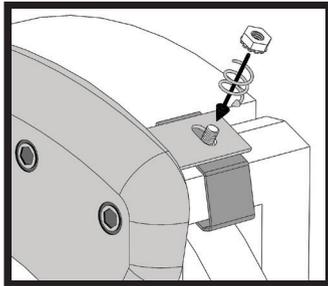
Install the supplied locknuts onto the threaded studs to secure bridge to clip. Tighten with 3/8-inch wrench or socket to 25 inch-pounds. Over tightening could pull stud through aluminum bridge.
