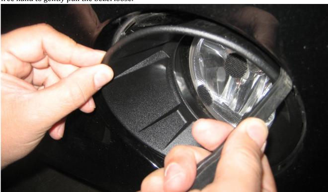
$Step\ Four: \ {\tt Pull\ out\ the\ factory\ bezel\ once\ it\ is\ free\ from\ the\ vehicle}.$
