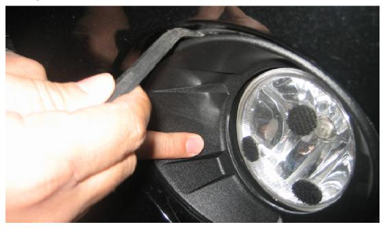
**Step Two:** Once the flat head is inserted into the bezel, slide prior into factory bezel and create a separation pocket.
