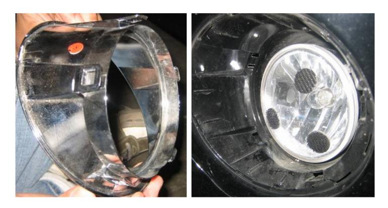
**Step Seven:** Insert the DefenderWorx Chrome Running Light Bezel into the crevice. Attachment clips should press firmly into place.
