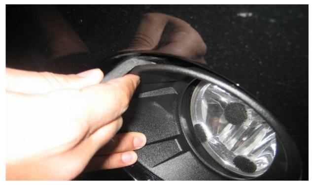
**Step Three:** Slide the flat head around the edges of the factory bezel and use your free hand to gently pull the bezel loose.
