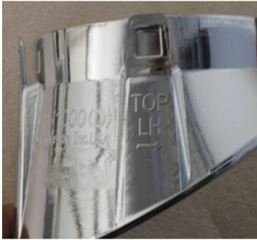
**Step Six:** Align the DefenderWorx Chrome Running Lights Bezel's attachment clips to the inside of the vehicle's crevice.
