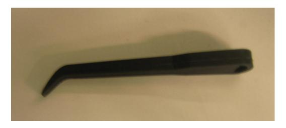
**Step One:** Insert rubber flat head into the factory bezel. Make sure to use a **Plastic** Flat head to prevent scratches.
