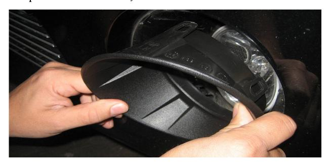
**Step Five:** The Bezel that reads, "Top RH" is for the passenger side of the vehicle, and the bezel that reads "Top LH" is for the driver's side.
