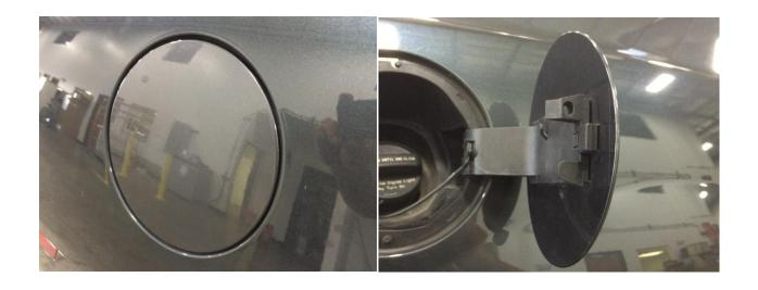
2. Using your right hand, wrap your fingers around the edge of the fuel door closest to the car body when in the open position. With your left thumb, pull the plastic retaining clip slightly away (to the left as you face the car with the fuel door open). Now pull with your right hand toward your body. The fuel door should slide along the hinged inner door toward you about ¼ inch and then to the right and off the hinged inner door.
